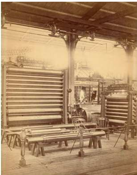
A photo from the 1876 Centennial Exhibition Digital Collection, showing J. Morton Poole's exhibit of calender rolls in Machinery Hall.
